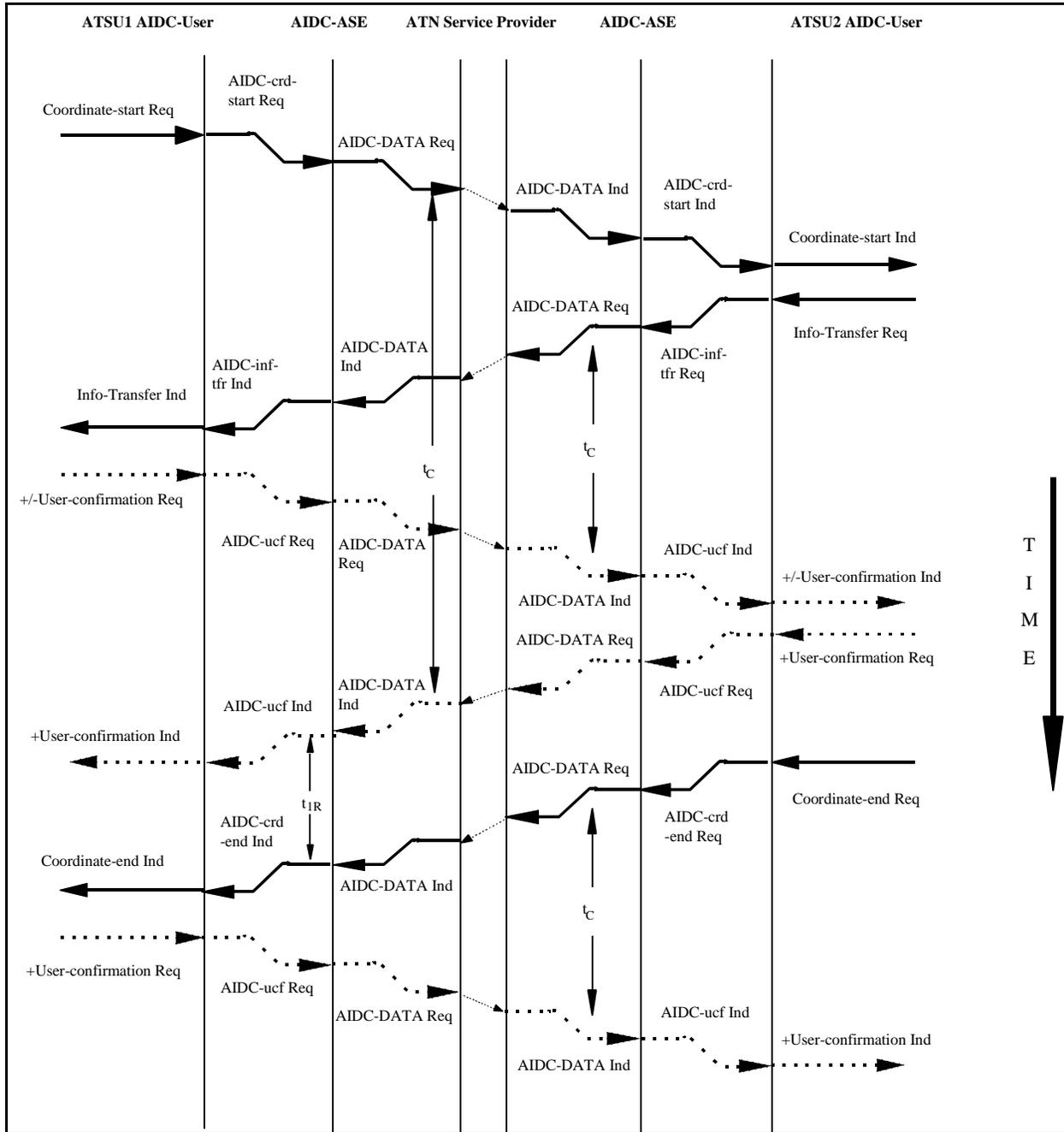
Figure 3.2.10-24: Sequence Diagram showing the invocation of the Info-transfer service before the User Confirmation of the Coordinate-start service
