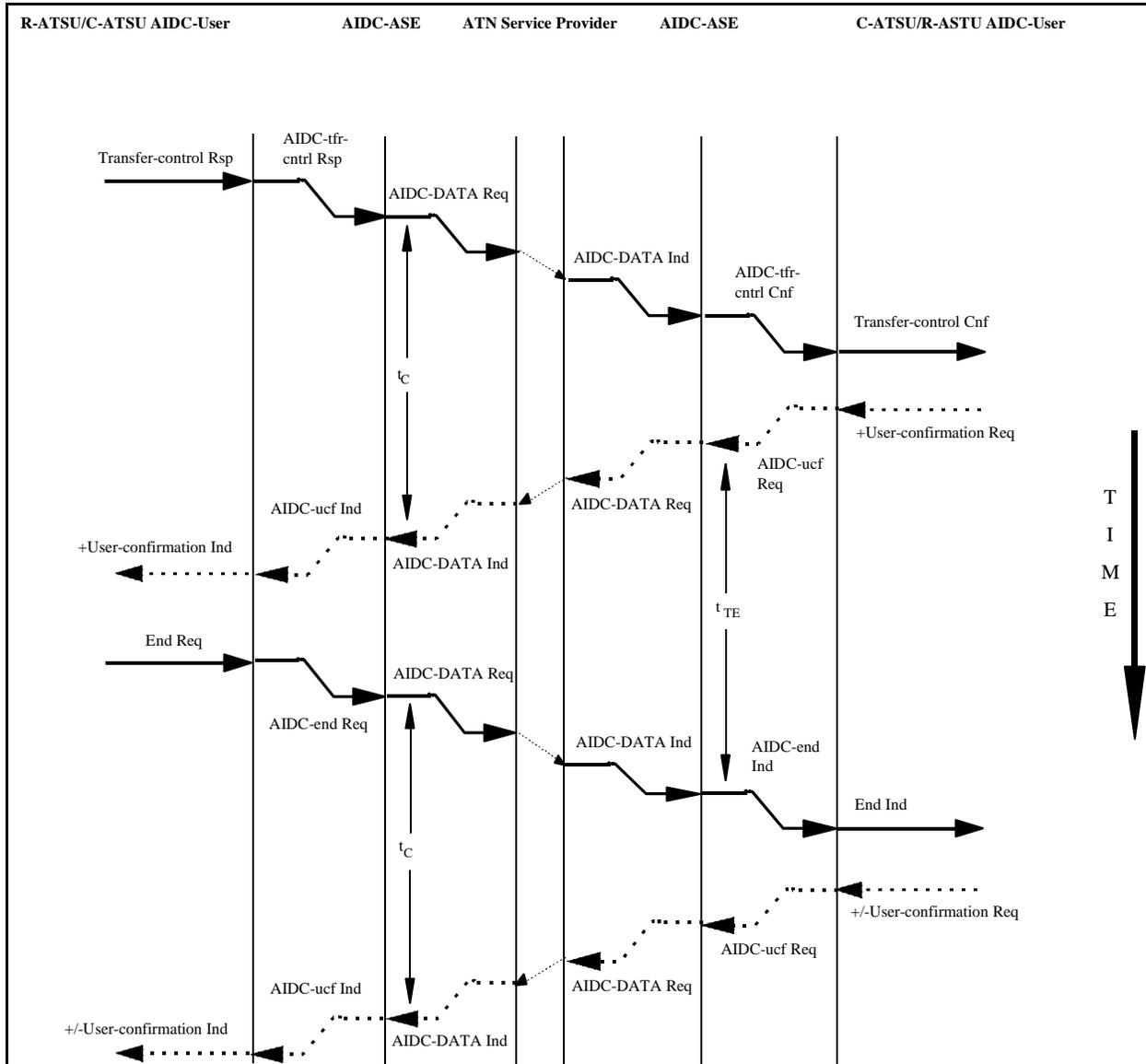
**Figure 3.2.10-21: Sequence Diagram showing the end of the AIDC service after the Transfer-control service**
