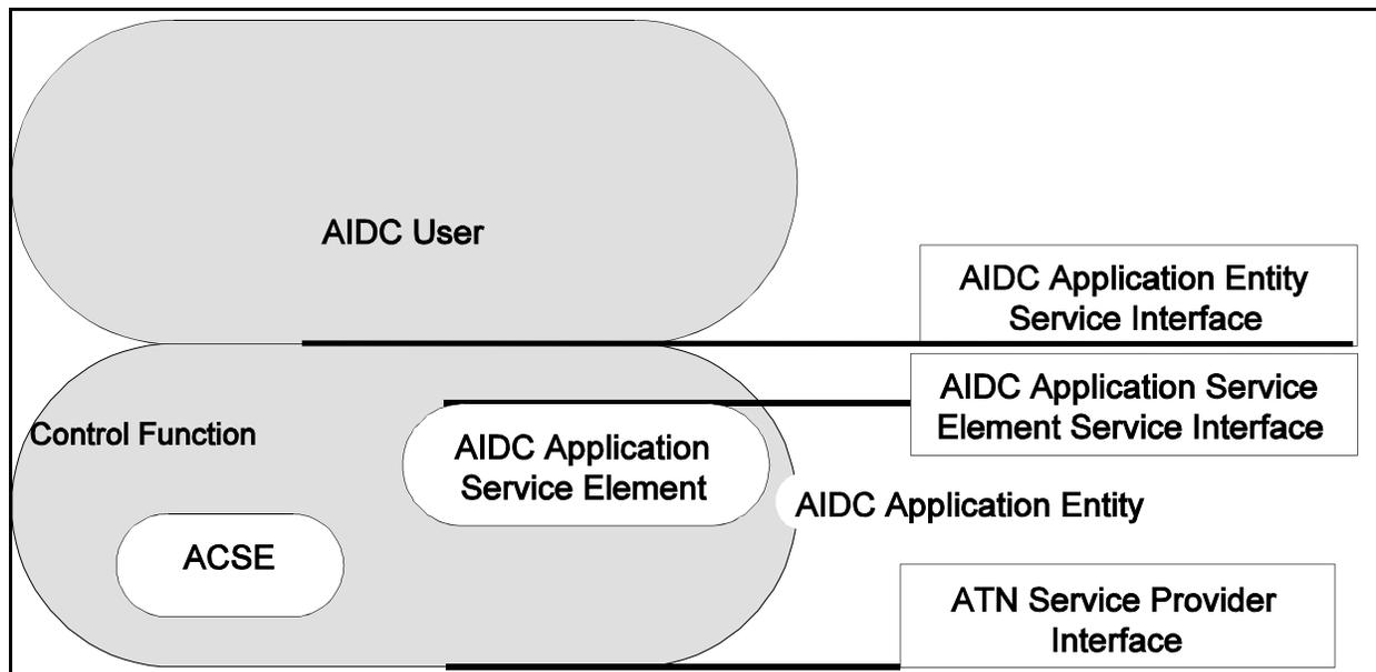
**Figure 3.2.1-1: Functional Model of the AIDC Application**
