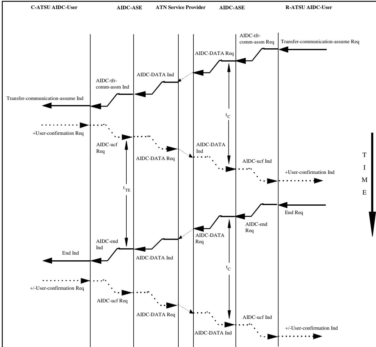
Figure 3.2.10-18: Sequence Diagram showing the end of the AIDC service through the invocation of the End service after the Transfer-communication-assume service
