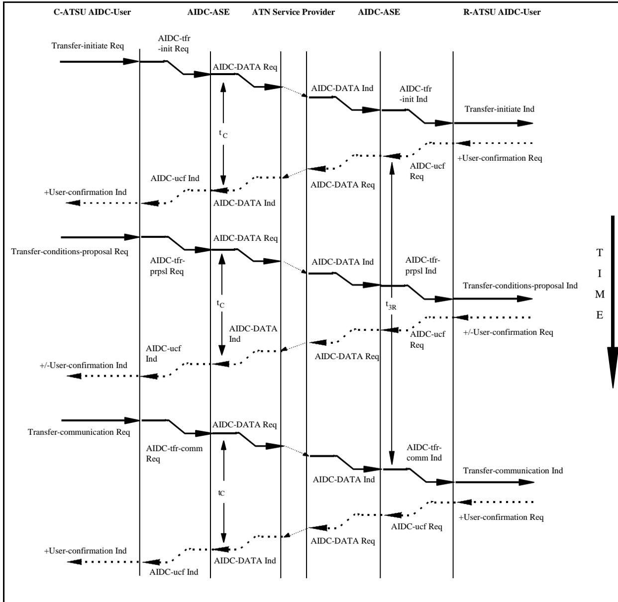
Figure 3.2.10-14: Sequence Diagram showing the invocation of the Transfer-conditions-proposal service, with predicate P1 false, followed by Transfer-communication service
