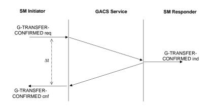
Figure 1. Simple confidence test and round trip measurement
