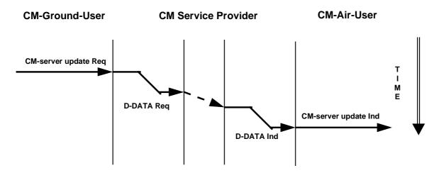
Note that although this service may be used if a dialogue does not exist, the CM-grounduser must not be allowed to invoke this service without knowing for sure what CM version the aircraft is carrying, or else an abort will occur. This is the same case as with the regular CM-update service.
