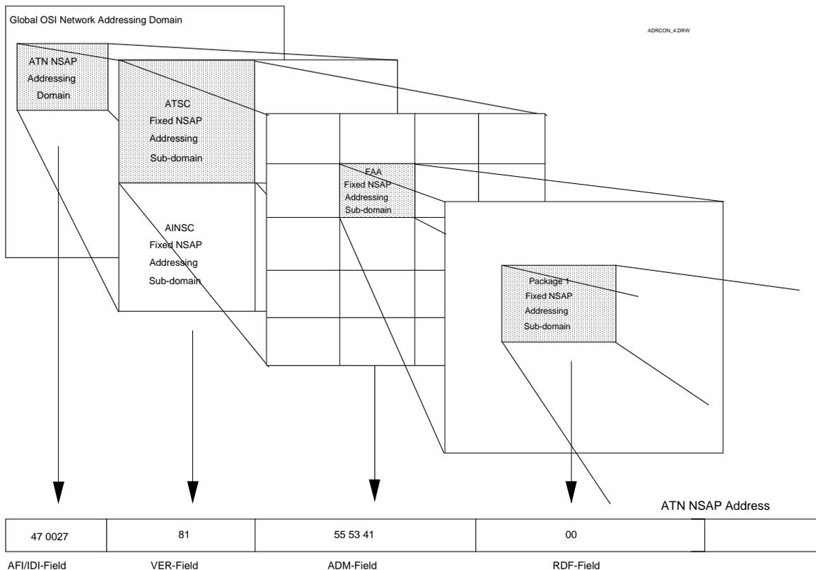
Figure 1: Hierarchical Decomposition of Addressing Domains Illustrated for ATN Network Addresses
