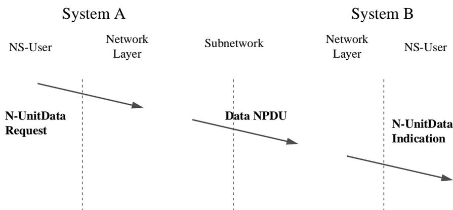
**Figure 4-1 Connectionless Network Service**
