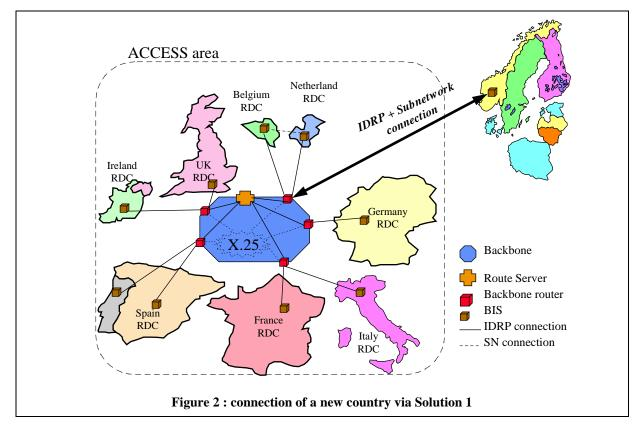
The interconnection between the router of the new country and the backbone router necessitates the attachment of both routers to a common subnetwork. If no suitable existing subnetwork is available, a possible solution is to use a leased line, which will then be dedicated to the ATN traffic between the 2 routers. Other solutions may be appropriate: e.g. use of a CIDIN connection, public X.25 networks, etc...
