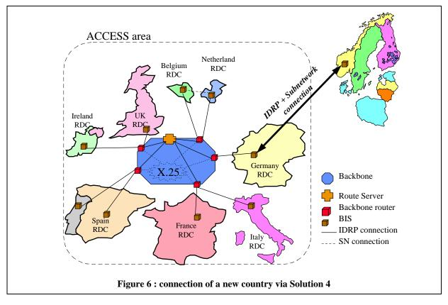
With this solution, the new ATN participant is not directly attached to the ATN backbone. Its international ATN traffic transits through the ATN infrastructure of the adjacent ATSO to which it is interconnected.
